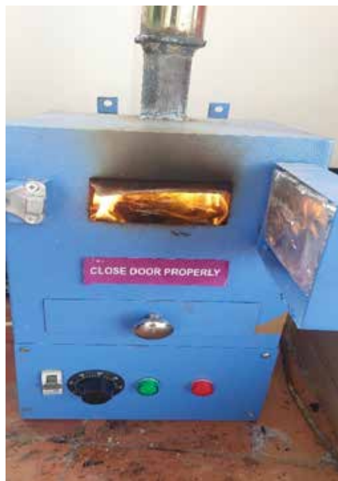
Figure 2: Small-scale incinerators showing a single chamber for burning the napkins and releasing the fumes from the top
