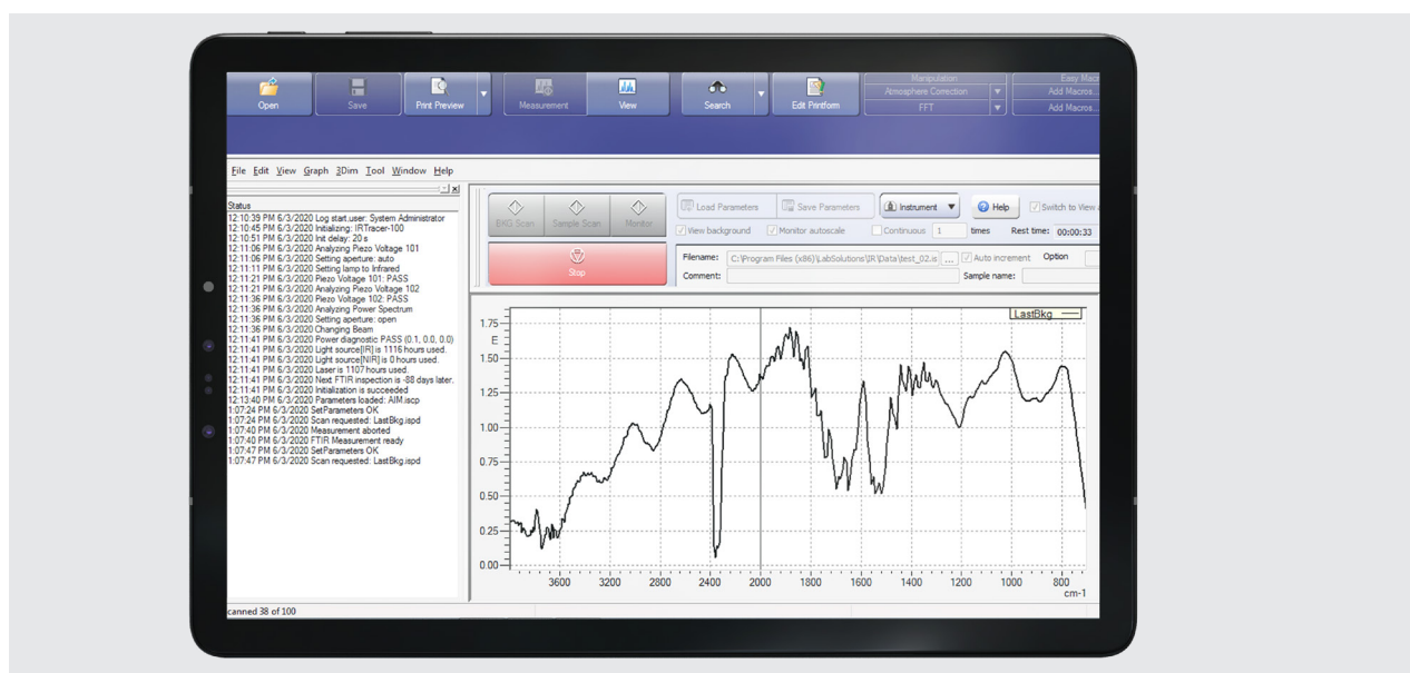
Figure 6: Background scan before analysis of MP samples in FTIR(IR Tracer- 100)
