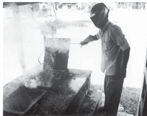
Primitive technologies such as De Montfort incinerators are operated in India under highly unsafe conditions.
