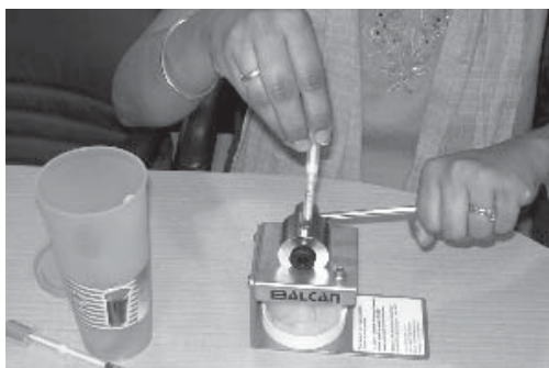
The Balcan cutter in use – the puncture-proof sharps container is seen to the left.
