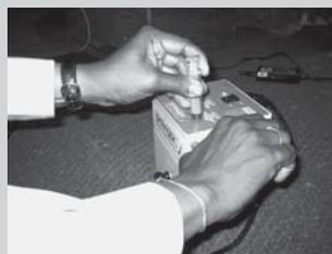
of carbon (usually 0.1% but as low as 0.03%). The purpose of the electric needle destroyer is to melt the iron alloy in the stainless steel needle.
