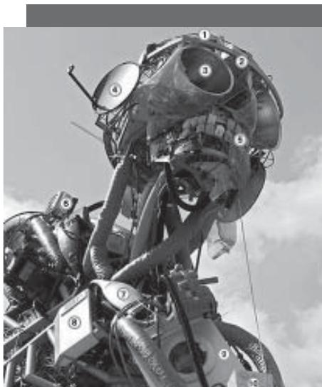
Components include: (1) PC screens; (2) printers; (3) industrial lights; (4) satellite dishes; (5) computer mice; (6) toasters; (7) vacuum cleaners; (8) heaters; (9) washing machines; (10) microwaves
